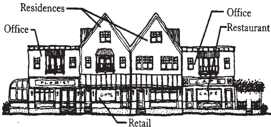
Example of a mixed-use development
