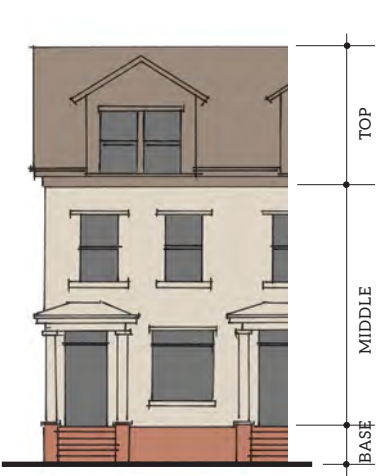
Figure 2.112 Building 2.5 stories or shorter broken down horizontally
