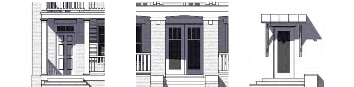
Figure 2.121 Examples of entry doors for multiple-family development
