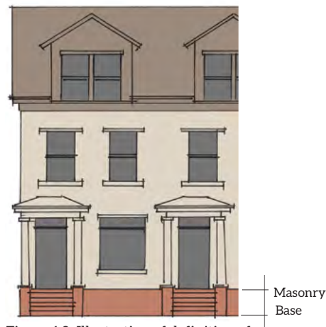
Figure 1.9 Illustration of definition of Masonry Base
