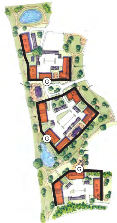
Figure 2.64 Building frontage at perimeter
