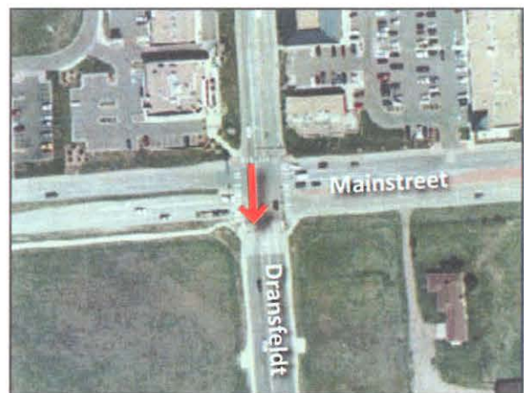
The red arrow through movement at Mainstreet and Dransfeldt Road has insufficient capacity.
