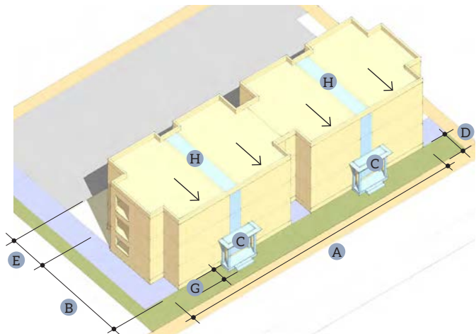
Figure 2.88 Example of Single-Aspect Walk-Up Multiple-Family Building
