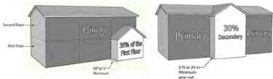
Figure 08.24 Elevation Plane Variation Requirement
