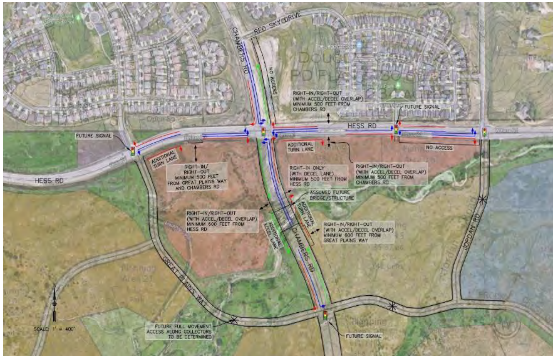
Figure 23 - Potential access locations in the study area. Source: David Evans & Associates.
