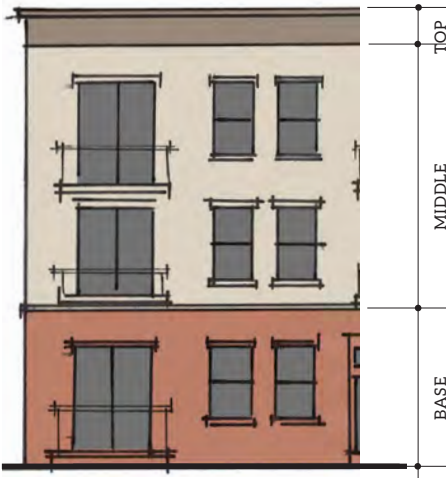
Figure 2.113 Building 3 stories or taller broken down horizontally
