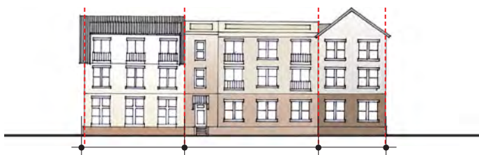
Figure 2.123 Composing a building as multiple buildings
