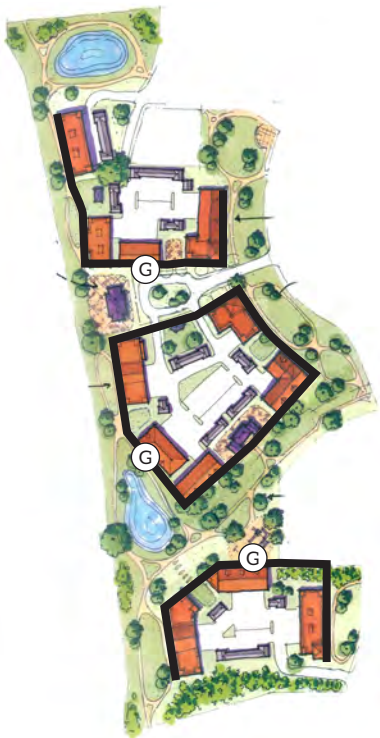
Figure 2.64 Building frontage at perimeter
