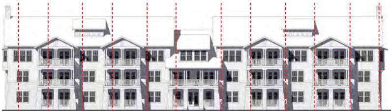
Figure 2.116 Walk-up Multiple-Family Building with regularly spaced bays
