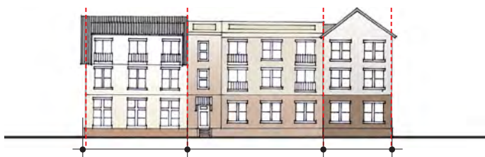
Figure 2.123 Composing a building as multiple buildings
