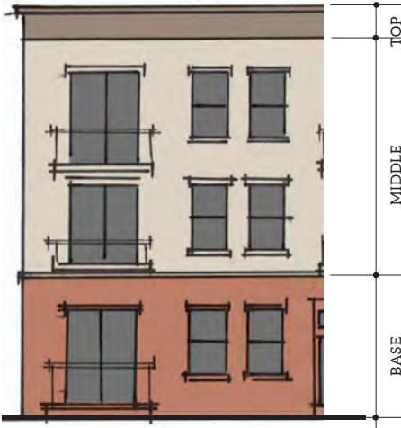
Figure 2.113 Building 3 stories or taller broken down horizontally
