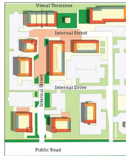
Figure 41 - Mixed-use site along an internal street.
